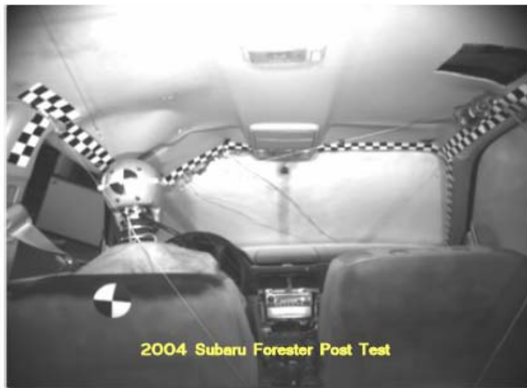
Far side 10° Pitch Intrusion w/ buckled header
